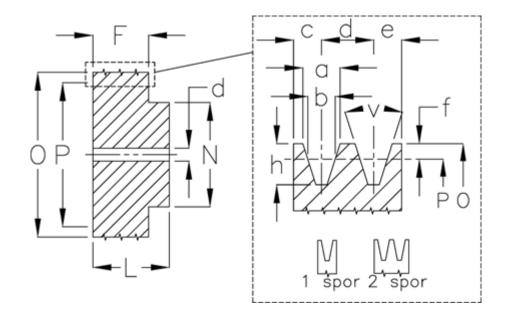
$\begin{array}{lll} d & = 10 \\ F & = 16 \\ L & = 28 \\ N & = 40 \\ Number of ribs = 1 \\ O & = 54.0 \\ P & = 50 \\ Type & = S \end{array}$
